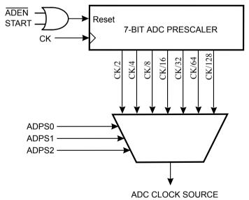
By default, the successive approximation circuitry requires an input clock frequency between 50kHz and 2MHz to get maximum resolution. If a lower resolution than 10 bits is needed, the input clock frequency to the ADC can be higher than 2MHz to get a higher sample rate.
