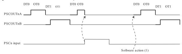
Note: Software action is the setting of the PRUNn bit in PCTLn register.
