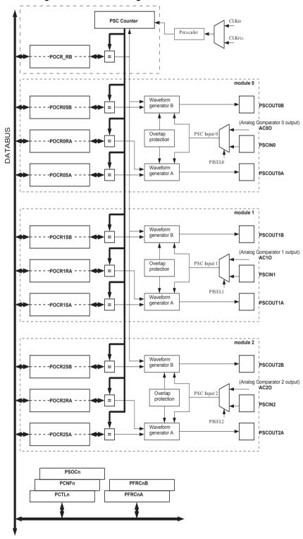
The PSC is based on the use of a free-running 12-bit counter (PSC counter). This counter is able to count up to a top value determined by the contents of POCR\_RB register and then according to the selected running mode, count down or reset to zero for another cycle.
