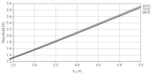
Figure 30-8. I/O pin input threshold voltage versus V<sub>CC</sub>. VIL, I/O pin read as '0'.
