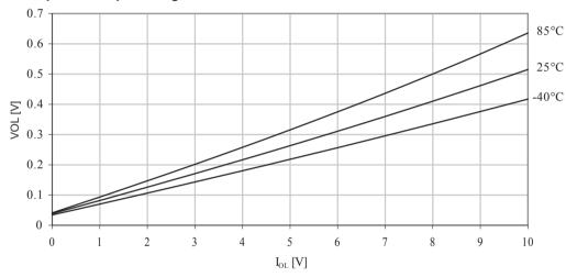
Figure 30-5. I/O pin output voltage versus source current. VCC = 5V.
