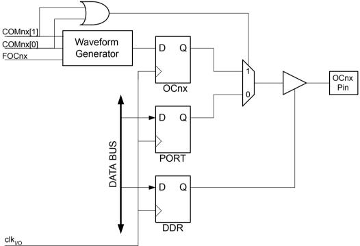
**Note:** The "n" in the register and bit names indicates the device number (n = 0 for Timer/Counter 0), and the "x" indicates Output Compare unit (A/B).
