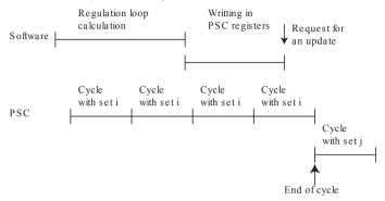
The software can stop the cycle before the end to update the values and restart a new PSC cycle.
