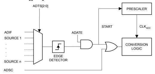
Using the ADC Interrupt Flag as a trigger source makes the ADC start a new conversion as soon as the ongoing conversion has finished. The ADC then operates in Free Running mode, constantly sampling and updating the ADC Data Register. The first conversion must be started by writing a '1' to ADCSRA.ADSC. In this mode the ADC will perform successive conversions independently of whether the ADC Interrupt Flag (ADIF) is cleared or not. The free running mode is not allowed on the amplified channels.
