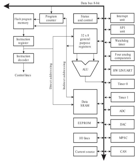
The AVR core combines a rich instruction set with 32 general purpose working registers. All the 32 registers are directly connected to the Arithmetic Logic Unit (ALU), allowing two independent registers to be accessed in one single instruction executed in one clock cycle. The resulting architecture is more code efficient while achieving throughputs up to ten times faster than conventional CISC microcontrollers.
