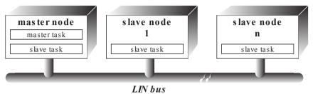
The master task decides when and which frame shall be transferred on the bus. The slave tasks provide the data transported by each frame. Both the master task and the slave task are parts of the Frame handler.
