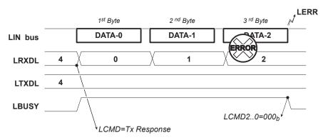
**Note:** Information on response (ex: error on byte) is only available at the end of the serialization/deserialization of the byte.
