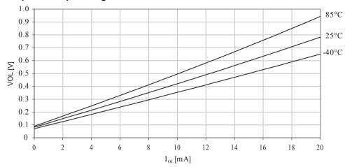
Figure 30-4. I/O pin low output voltage versus sink current. VCC = 3V.
