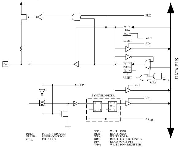
Note: 1. WRx, WPx, WDx, RRx, RPx, and RDx are common to all pins within the same port.  $clk_{I/O}$ , SLEEP, and PUD are common to all ports.
