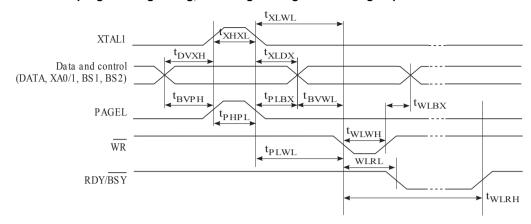
Figure 29-6. Parallel programming timing, loading sequence with timing requirements.
