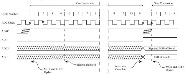
Figure 22-6. ADC Timing Diagram, Auto Triggered Conversion
