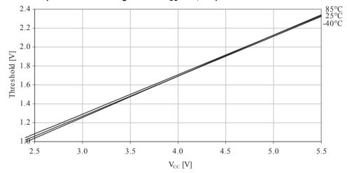
Figure 30-11. Reset input threshold voltage versus  $V_{\text{CC}}$ . VIL, I/O pin read as '0'.
