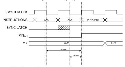
Consider the clock period starting shortly after the first falling edge of the system clock. The latch is closed when the clock is low, and goes transparent when the clock is high, as indicated by the shaded
