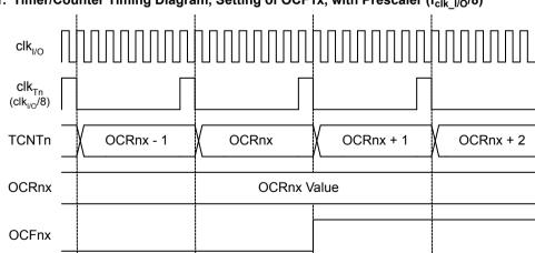
Figure 16-11. Timer/Counter Timing Diagram, Setting of OCF1x, with Prescaler (f<sub>clk I/O</sub>/8)
