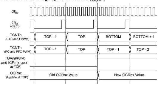
Figure 16-13. Timer/Counter Timing Diagram, with Prescaler (f<sub>clk I/O</sub>/8)
