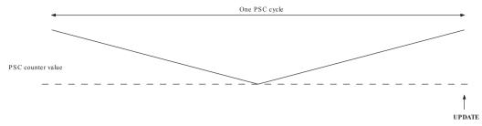
The figures above graphically illustrate the values held in the PSC counter. Centered mode is like One Ramp mode which counts down and then up.
